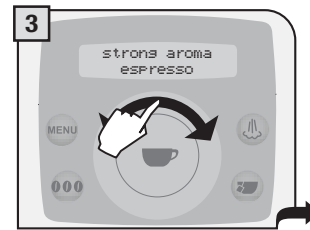
3 Select the desired beverage by navigating the click wheel with your finger.
